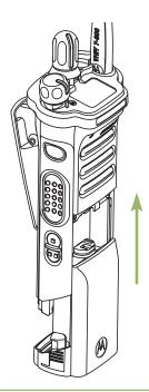
2 To remove the battery, squeeze the release latches (A) at the bottom of the battery until the battery releases from the radio and remove the battery from the radio.
